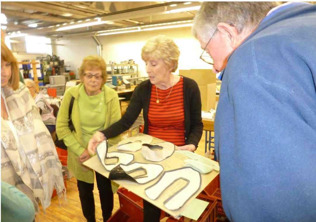
Avis explaining the cutting out of the leather Uppers and their stitching
